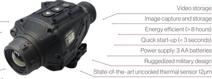
SENSORS THERMIS MK2 family of uncooled Thermal Sights was developed to provide soldiers with an unrivaled day / night advantage in detecting, observing and engaging hostile targets, independent of darkness and common obscurants used for visual concealment
